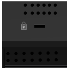
Figure 2-3 A Typical Kensington Lock
